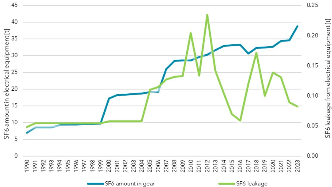
Figure 4.6 Total SF<sub>6</sub> amounts contained in and SF<sub>6</sub> leakage from electrical equipment [t].
